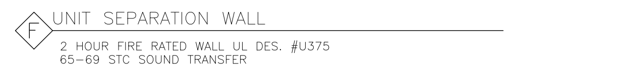
F UNIT SEPARATION WALL
