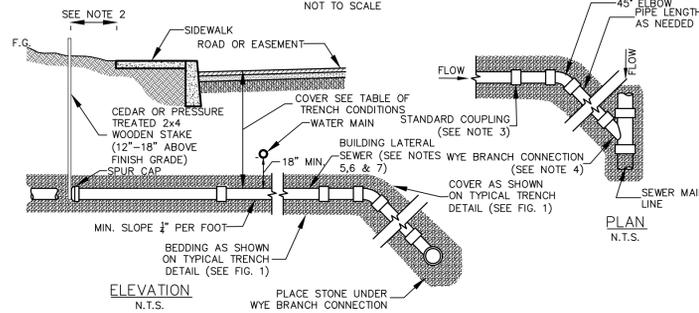
**SANITARY SEWER SPECIFICATIONS (FOR BUILDING LATERAL SEWERS AND SEWER MAIN LINE):**
