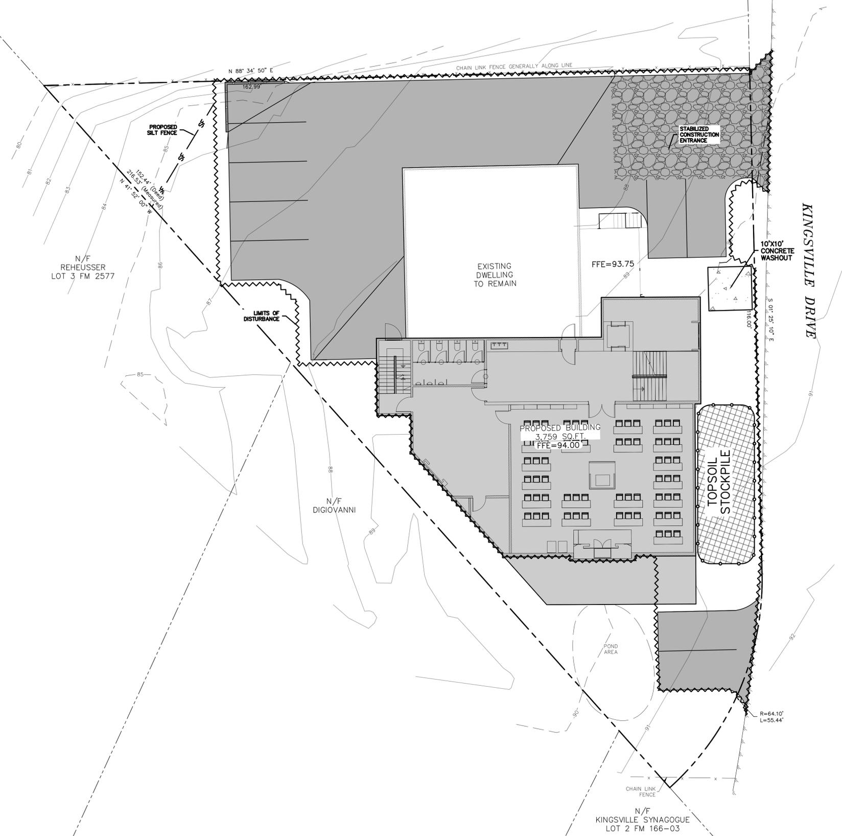
**06 EROSION AND SEDIMENT CONTROL PLAN**
