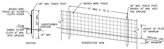
**CONSTRUCTION NOTES FOR FABRICATED SILT FENCE**
